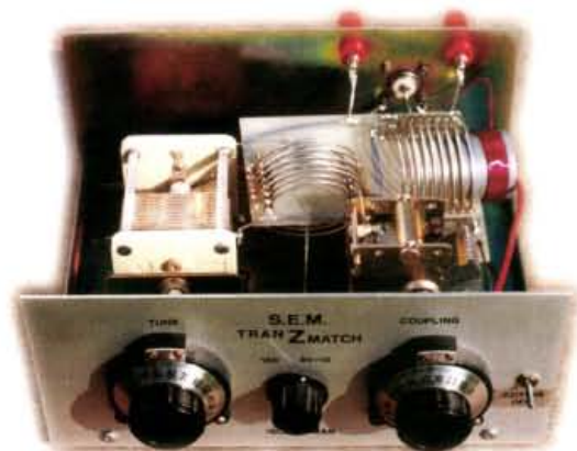
Fig. 4: The S.E.M. 'Transmatch' matching unit, which shows the general construction of a Z-match a.t.u.
